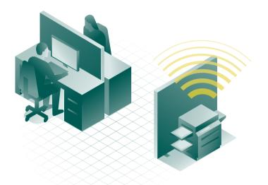
Ideally, acoustic screens should be placed close to workstations. This allows them to both shield the individual worker from incoming noise and absorb sound generated from the workstation. For the best effect one acoustic screen should be installed for every two workstations.
