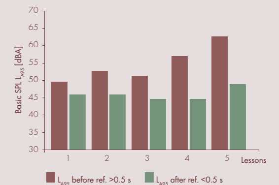
Increase of activity sound levels ( L_{A95} ) before and after refurbishment 3
